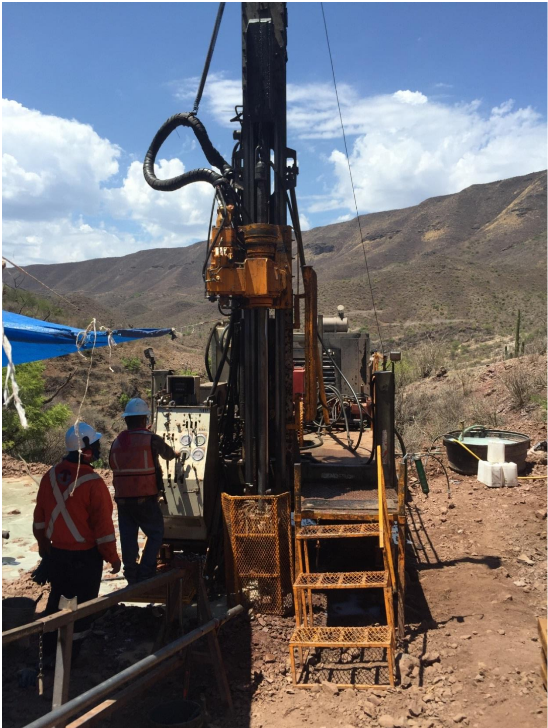
Figure 10.1.1: 2016 Toro Drilling Rig Producing NQ Drill Core
