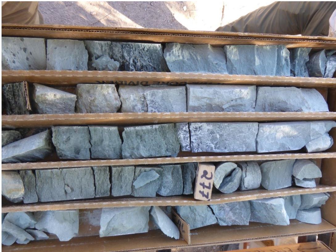
Figure 11.1.2: Drill Core Presented After Cut and Sampling Procedures
